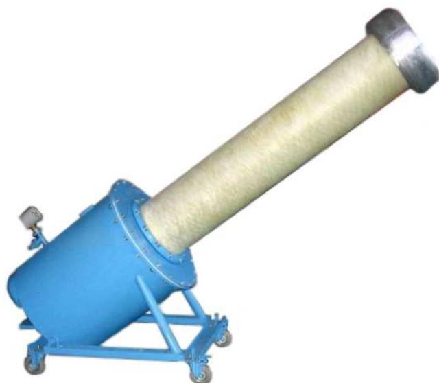
Single-phase gas-filled test transformer (IOG-200-II) is designed for testing electric switching module and conditioning vacuum arc chutes. The transformer can also be used for testing other electrical equipment with short-term 50 Hz high voltage.
