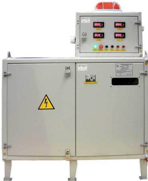
Oil-filled stationary high-voltage test installation UVISM-12 is designed for testing dielectric strength of insulation of direct and pulsating current traction motors and also asynchronous motors with voltage of 50 Hz frequency. It can be also used for high-voltage tests of 50 Hz frequency of other objects with appropriate voltage and capacity parameters.
