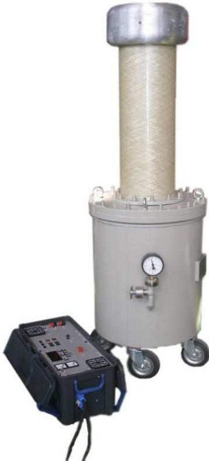
Gas-filled stationary test installation UISG-100-I is designed for 3,3 - 110 kV surge arresters testing under partial discharges level index
