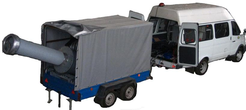
Gas-filled mobile test installation UVPG-250 is designed for tests of electrical equipment insulation with power frequency voltage of up to 250 kV inclusive. Owing to a low level of self-partial discharges (PD) it can be used for testing insulation with PD measurement at voltage of up to 200 kV inclusive.
