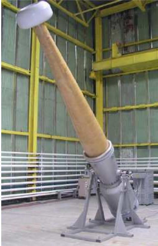
Gas-filled stationary test installation UISG-560 is designed for conducting tests of electrical equipment insulation with short-term 50 Hz high voltage, including tests with measuring capacitance ( $C_x$ ) and loss-angle tangent ( $\text{tg } \delta_n$ ) and partial discharges (PD).
