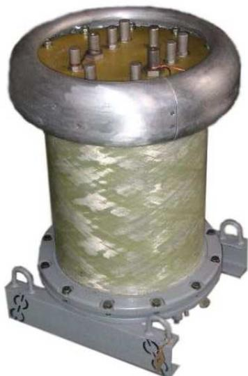
Separately mounted gas-filled current transformer (TOG-35-II) is designed for application as a mean of verification of industrially produced current transformers, can be used for transmission of the measuring information signal onto the measuring instruments during high-voltage tests of electrical equipment.
