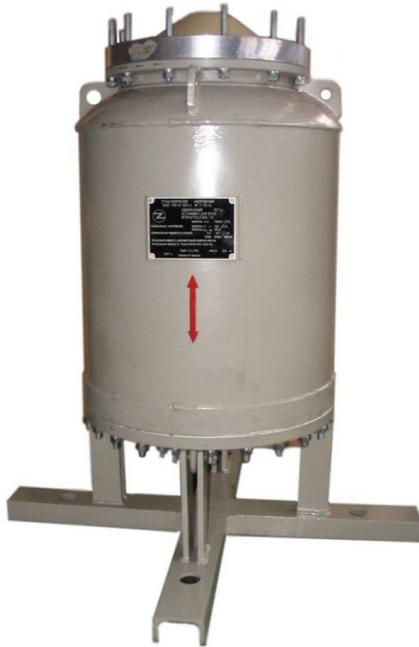
Voltage transformers of ZNOG-110 type are designed for use in switchgears and control gears with SF<sub>6</sub> insulation of 110kV voltage class, being installed in the mains with efficiently grounded neutral for feeding of the electric measuring devices, security circuits, warning and also as test transformers with the feeding from the side of the secondary windings.
